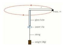
Circular motion can be investigated experimentally by tying a bung, with mass *m*, to a piece of string, and threading it through a glass tube. The other end of the string has a weight, with mass *M*, suspended from it. This provides the centripetal force, F = Mg, as the tension throughout the string is constant. The string is whirled in a circle, and the time taken for a complete rotation is recorded. The mass of the weight is altered and the experiment repeated.
